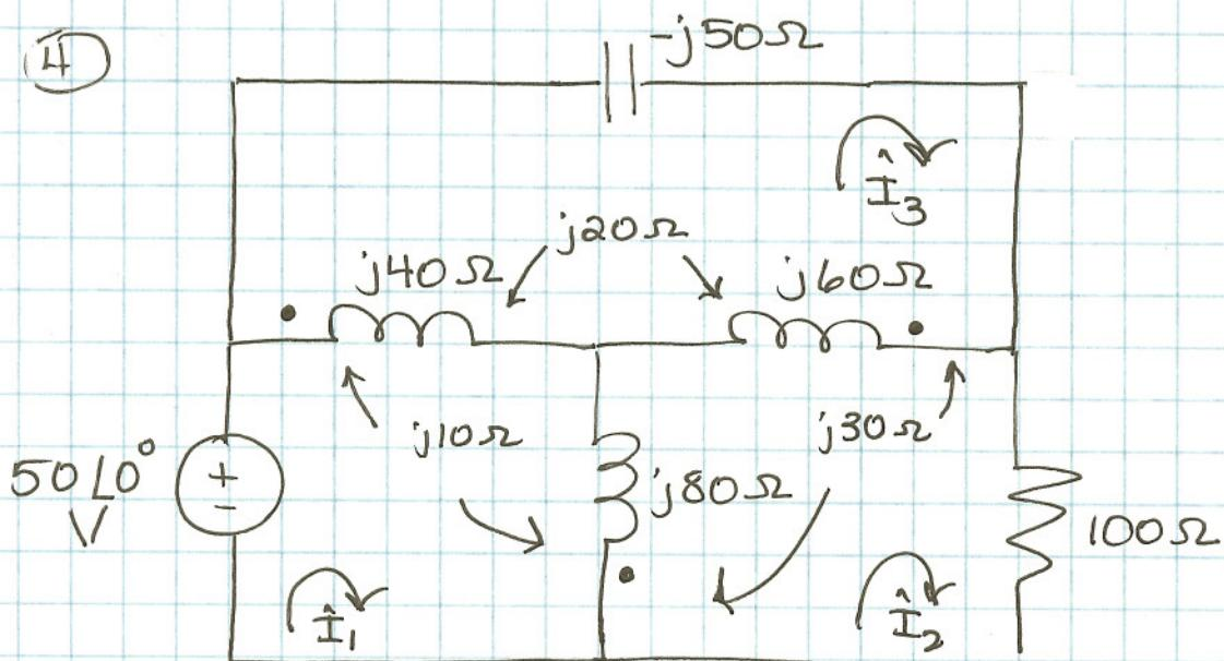
$$m_1: 50\angle 0^\circ - [j40(\dot{I}_1 - \dot{I}_3) + j10(\dot{I}_2 - \dot{I}_1) + j20(\dot{I}_3 - \dot{I}_2)] - \dots$$
