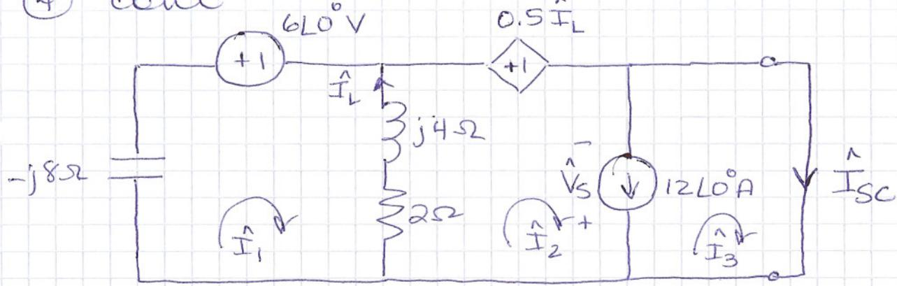
$$\text{Know } I_L = I_2 - I_1 \quad I_2 - I_3 = 12L0^{\circ}$$
