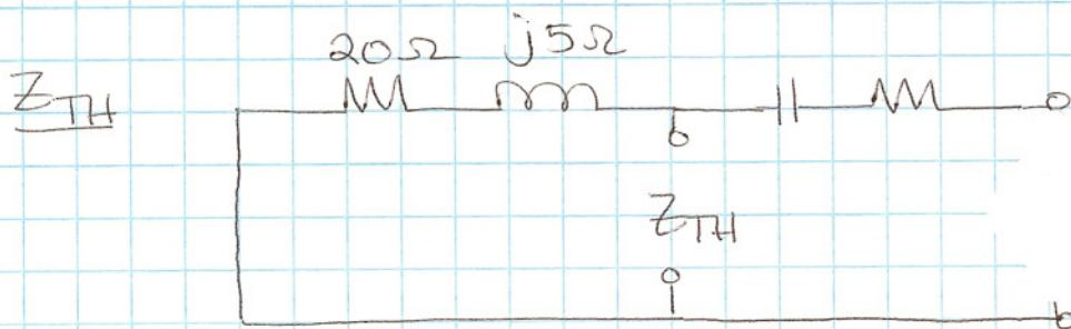
$$\underline{Z_{th}} = 20 + j5 \Omega \text{ or } 20.162 L 14.04^\circ \Omega$$
