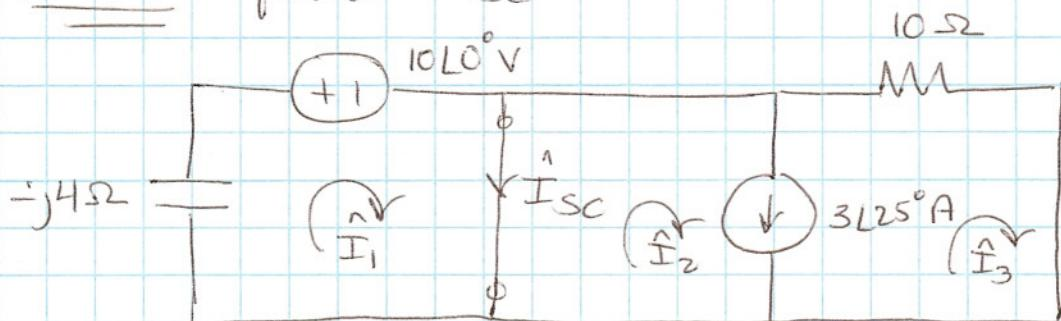
$$\begin{aligned} \text{know: } I_3 &= 0 \\ I_2 - I_3 &= 3L25^\circ \\ I_2 &= 3L25^\circ \end{aligned}$$
