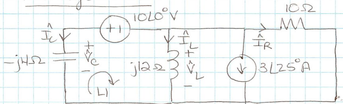
$$\text{for } \hat{I}_L = 1.99 L 85.15^\circ A \quad \hat{V}_L = j12 \hat{I}_L = 23.91 L 175.15^\circ V$$
