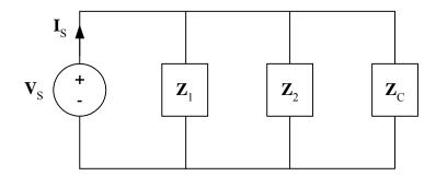
It is desired to add a new load in parallel with the other two loads, as shown above. The new load is to be designed to correct the power factor of the combined loads to 0.98 lagging. The real power delivered by the source, as well as the source voltage may not change. What is the impedance of the new load,  $Z_{\rm C}$ ?
