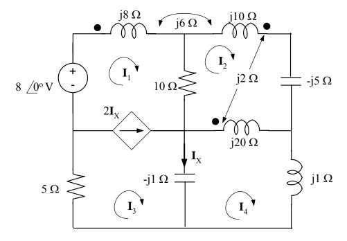
[20 points] Using the labeled mesh currents and directions, write down the four mesh equations (Do not simplify). Then write down any other equations required to solve the circuit (i.e. the number of equations equals the number of unknowns). Do not solve the equations.
