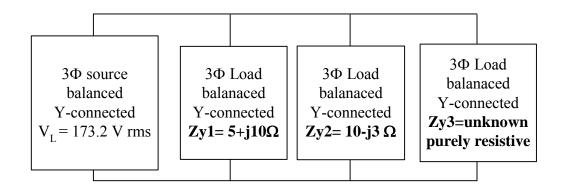
a. [10 points] Draw a block diagram of the single phase circuit of the three phase system labeled above. Make sure the label all pertinent voltages and currents and give the value of the line to neutral voltage,  $V_{an}$ .
