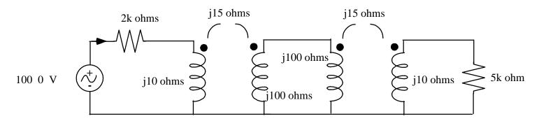
What is the power absorbed by the 5 k ohm resistor?
